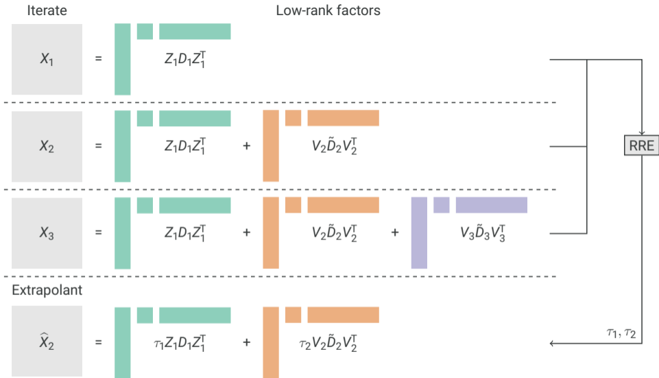
Figure: Increment-based RRE for low-rank matrix sequences, where \tau_i := \gamma_i + \dots + \gamma_n .
